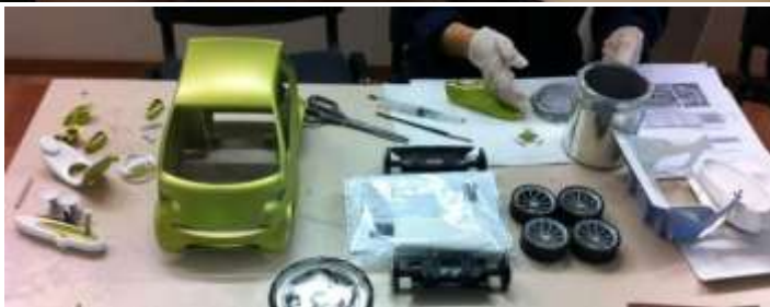
2010 Work project made in a course: Technical in Prototips in Fundacio CIM , UPC (Politechnic University of Catalonia, Barcelona), it consists in rebuild a car "smart" through 3d software as Catia and Solidworks and fabricate through 3d printers and different kind of molds
